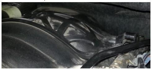
☐ Remove MAP and PVC lines from valve covers (drivers, passenger) and intake (front) – LS3 is different :
