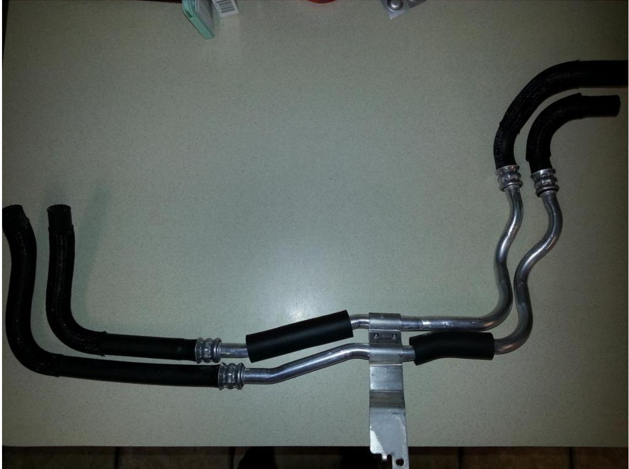
□ A 160\* thermostat can also be installed at this time (recommended, but not required) re-install the heater hoses @ this time if you relocated the heater hoses:
