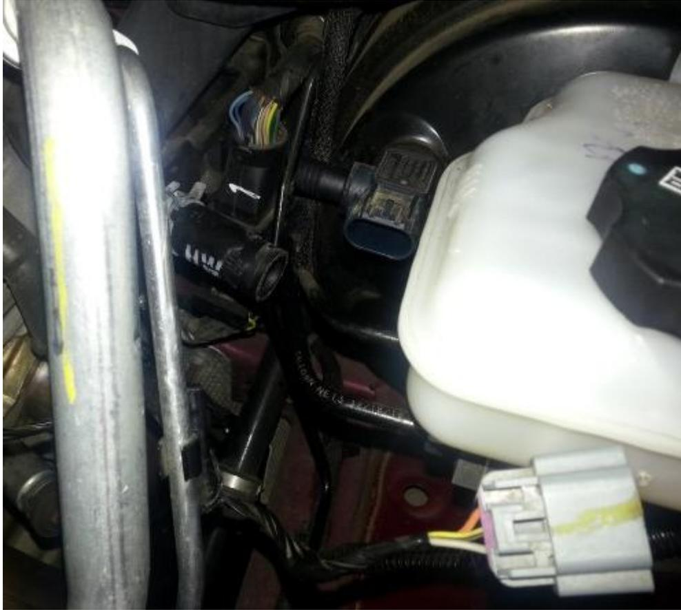
The L99 has a brake booster connector that you will also need to remove and mark the connector for re-assembly. The booster hose from the manifold is NOT re-used.
