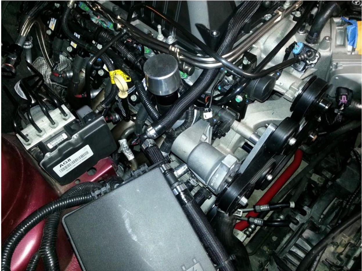
Tighten all hose clamps. Fill reservoir with 50/50 Dexcool. It will be necessary to 'milk' the lines to get the fluid through.
