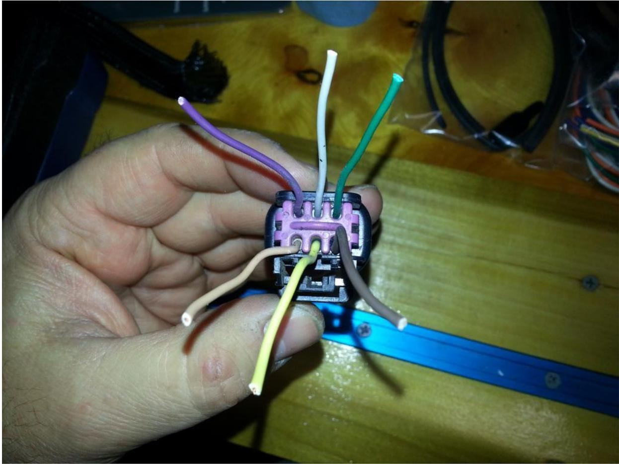
Now, using Rosin Core solders (60/40), begin by stripping the wire and soldering it. Also use the 'heat shrink tubes' to cover up the solder, then wrapped the sections of wire in electrical tape -- then finished off with the kit supplied wire cover (shrink wrap also):
