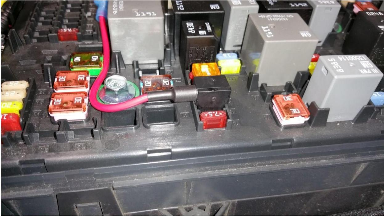
Tie-wrap the harness' and verify they don't pinch when the fuse box is closed:
