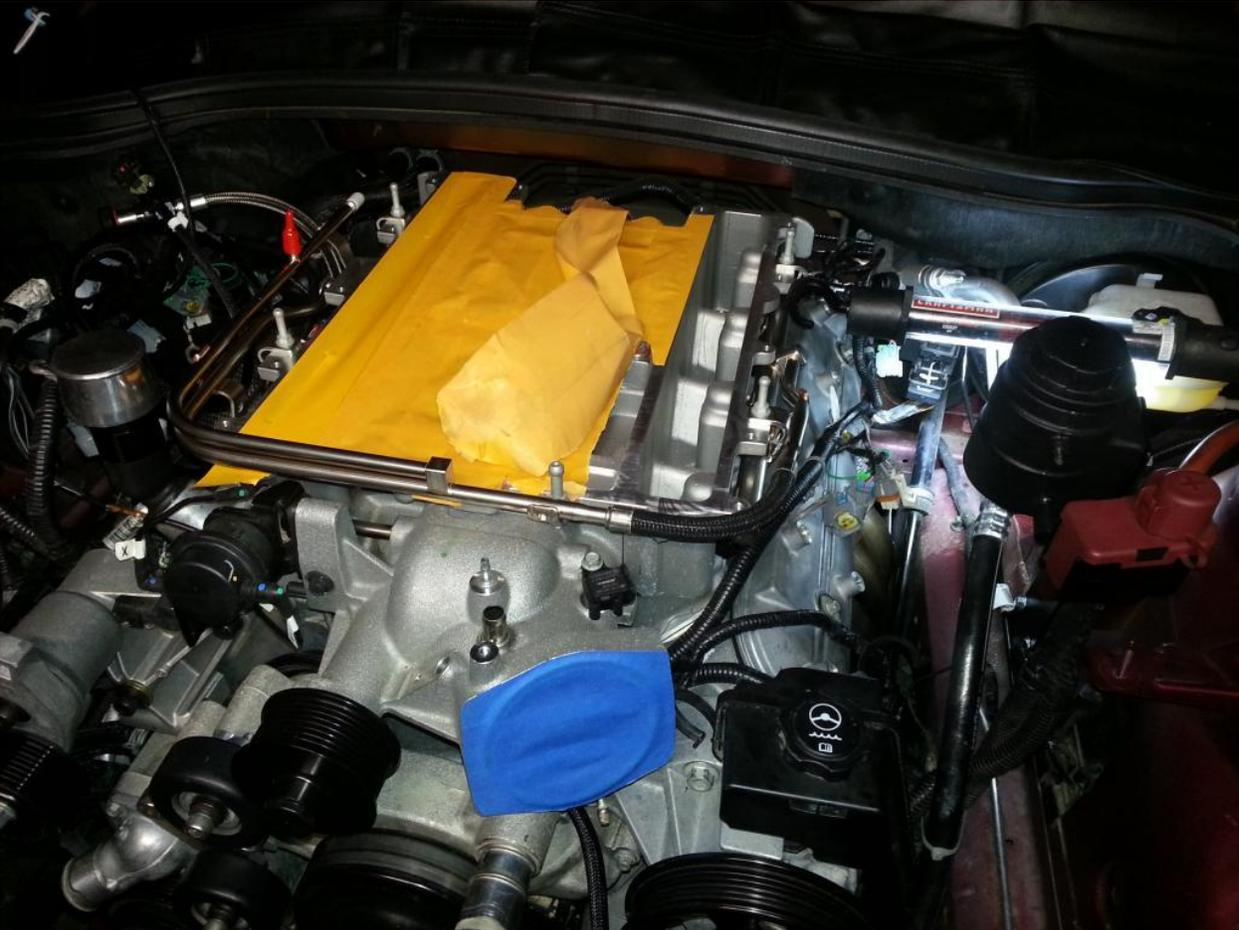
Make sure the wires are clear and not pinched by the Supercharger it will be necessary to 'ease' the steam tube down about 30 degrees to avoid hitting the manifold:
