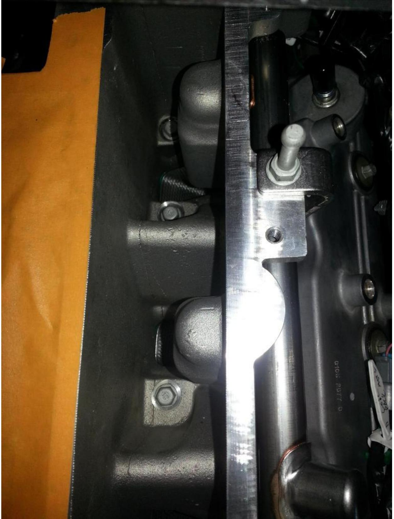
With the intake bolts torqued, cover up so nothing falls in until you are ready for the lid:
