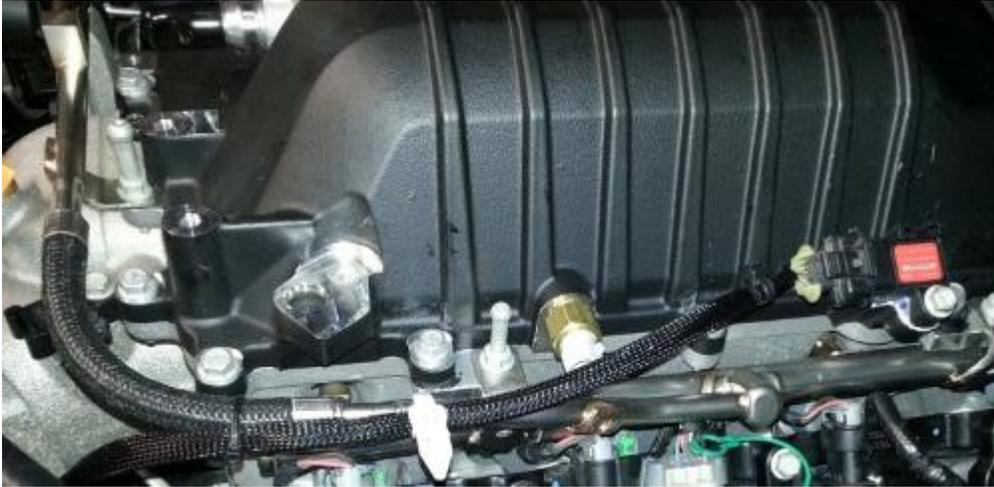
□ Install the brake booster hose (and connector if required), vacuum hoses to the manifold:
