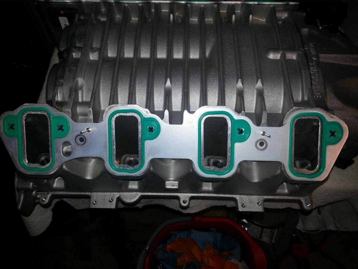
Make sure everything is centered up correctly (bolt holes) and rivet the NON-ELONGATED rivet first:
