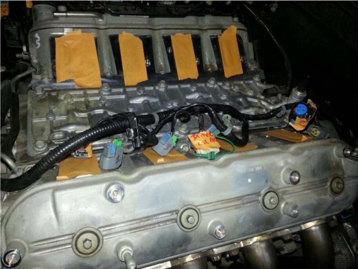
Note the bolt is 'raised' from the original location. You'll need to drill just above the existing hole:
