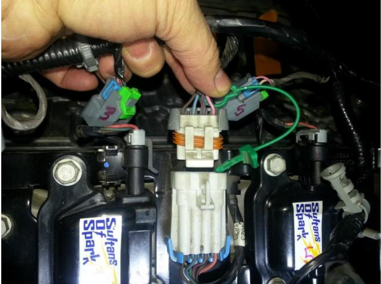
Unbolt coil packs and then drill the holes so you can 'lower' the coil packs for installation:
