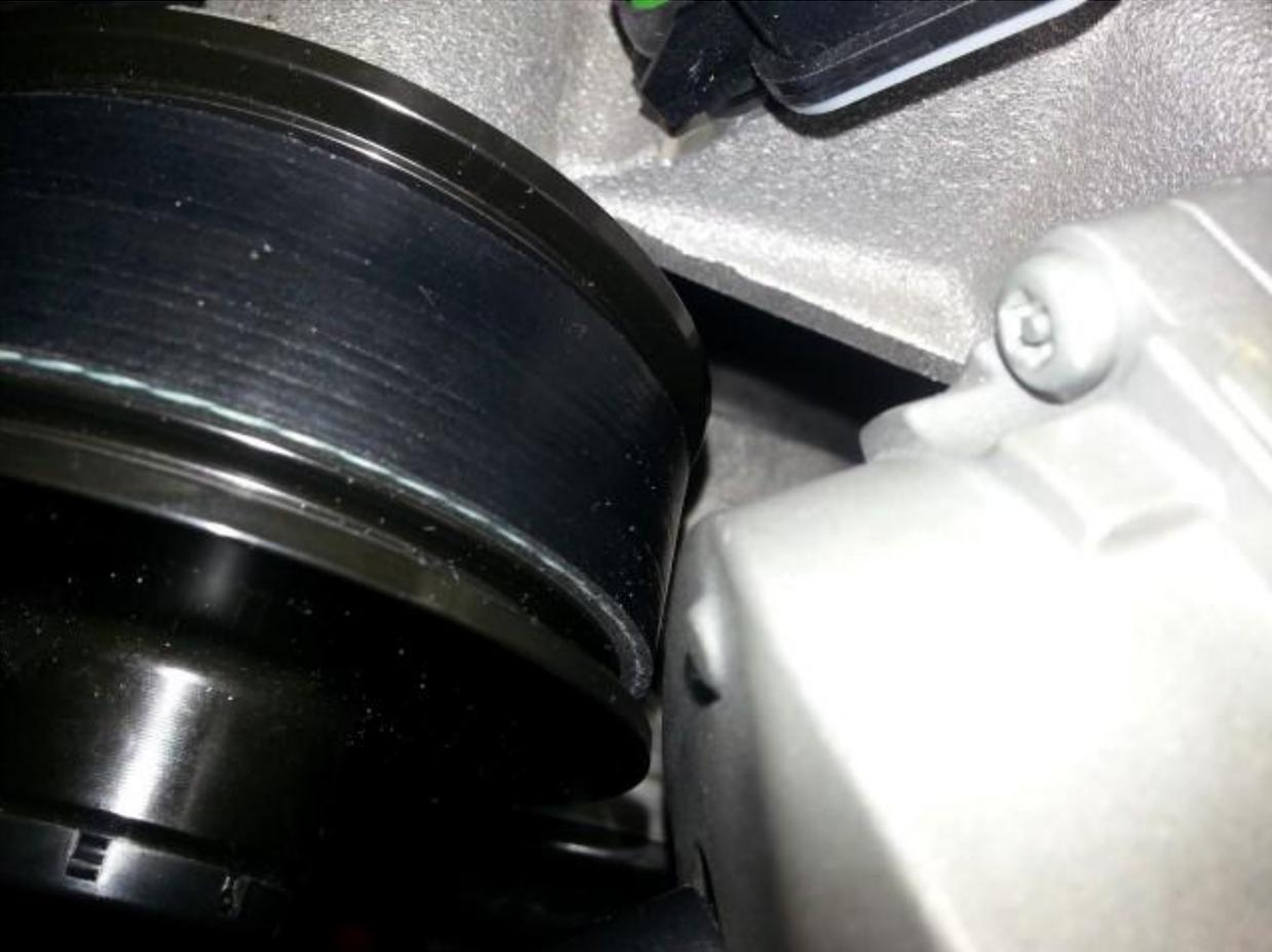
Connect the throttle body connector – make sure to route and avoid all pulleys:
