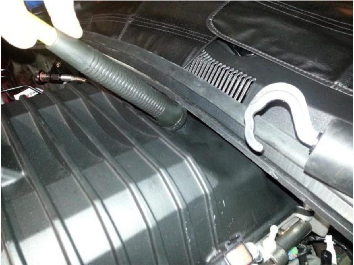
Reinstall the previously removed push pins back into the cowling.
