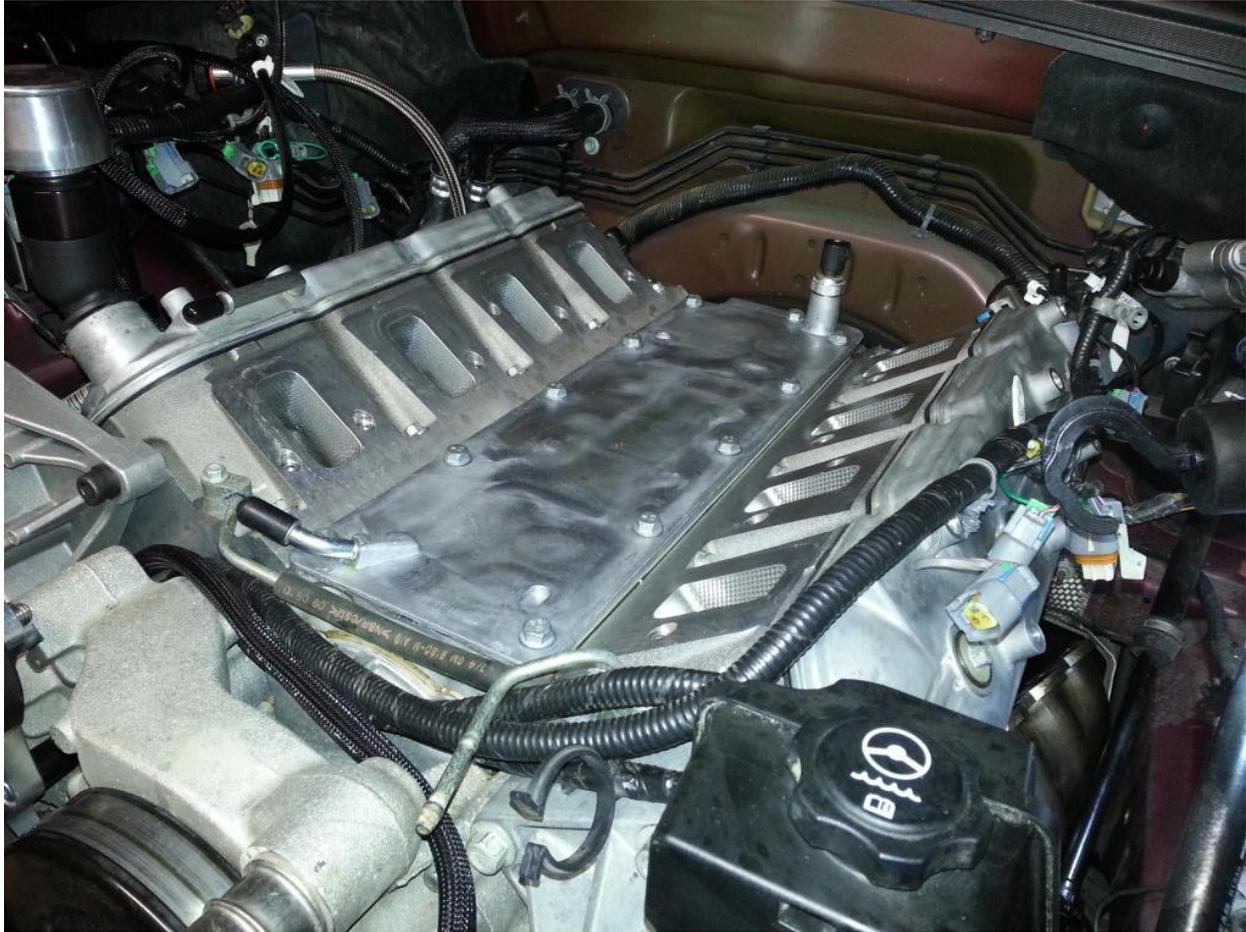
Lift the lower manifold onto the intake ports – this takes two people or a small 'lift':
