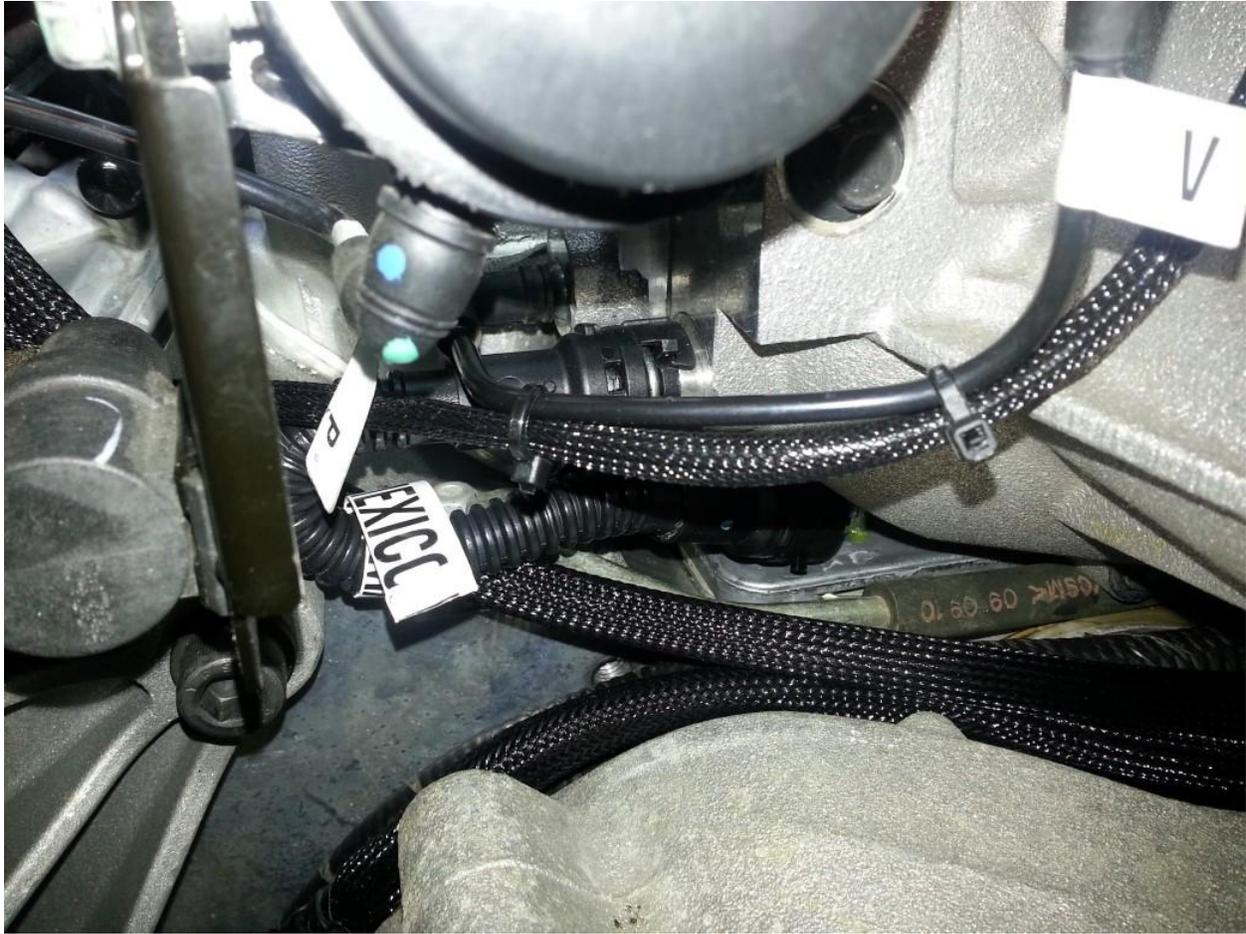
Verify all wires are clear of obstructions and all vacuum lines and PCV lines are hooked up:
