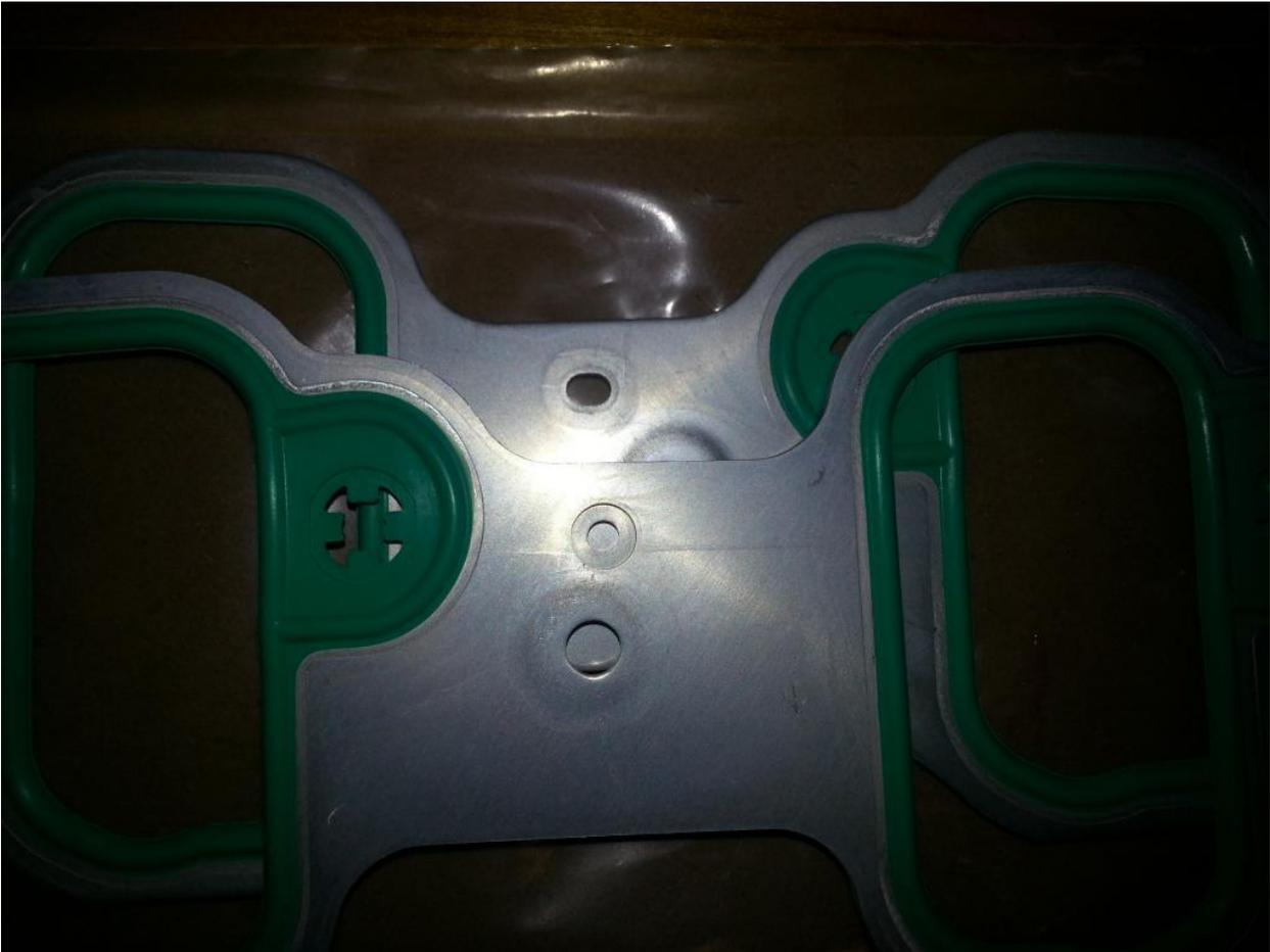
Place the rivets in the gaskets and set on manifold:
