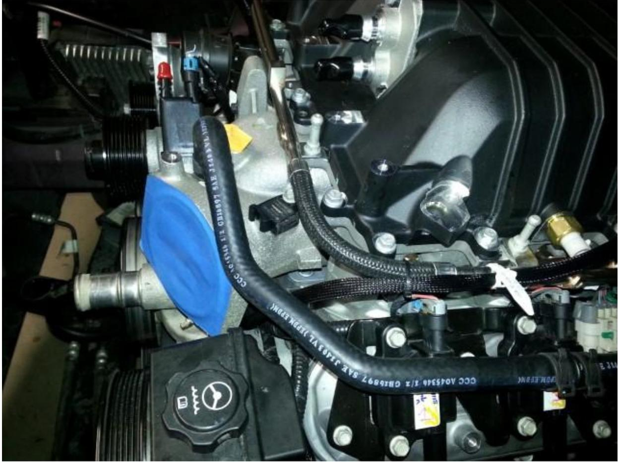
☐ Install Fuel and EVAP Lines to hard lines:
