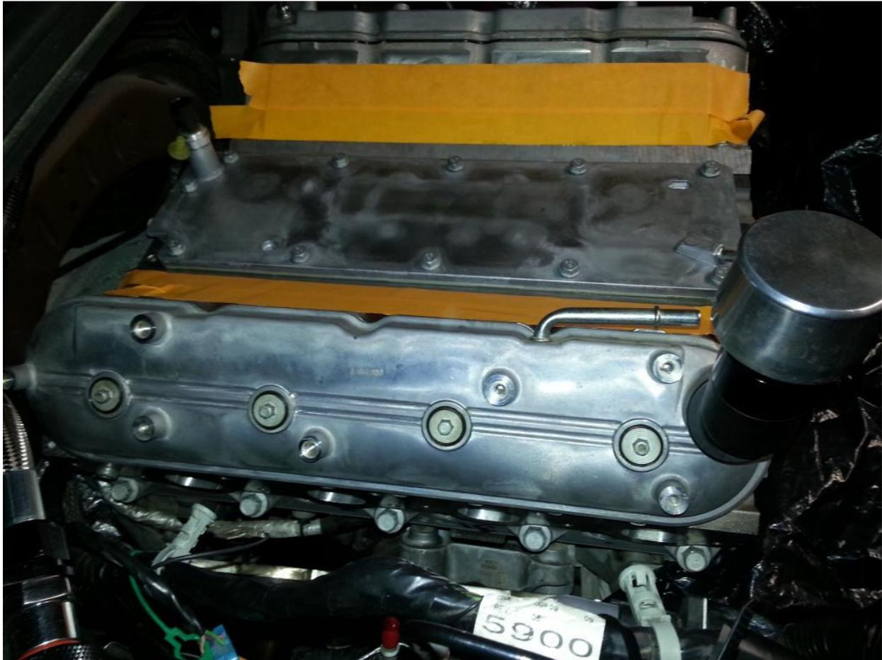
Valley cover bolts are torque to 18 ft. lbs., oil sender is 15 ft. lbs.
