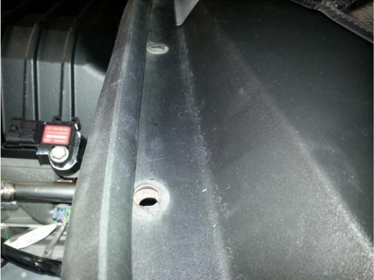
□ Using these types of tools, begin bolting down the lib (follow this sequence): To bolt down the # 15 and 16 bolts, you'll need to use a hammer handle (after you've tightened bolts 1-14) to give you better access:
