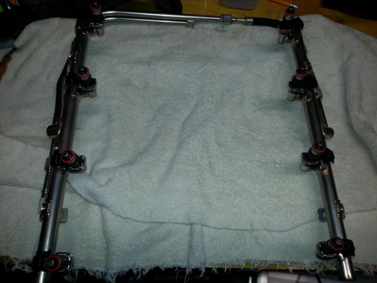
Installation requires you do the 'drivers' side injectors first to allow for the passenger's side to fit:
