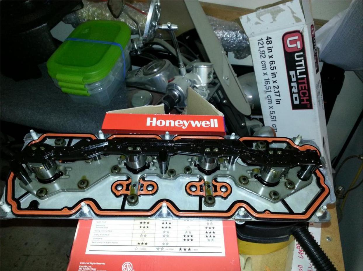
New valley cover with oil sending unit installed and bolted:
