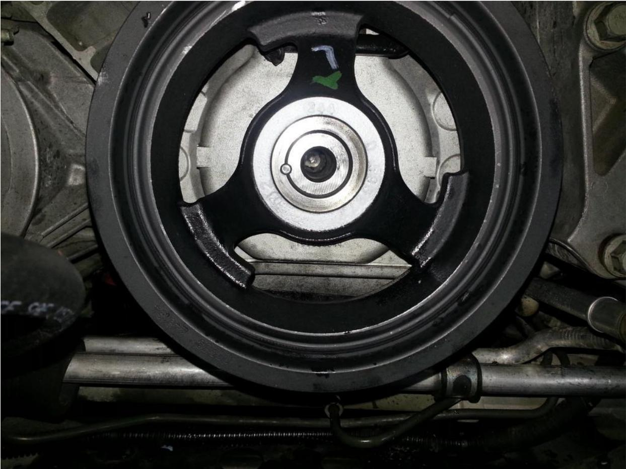
Bolted per pinning instructions (use red loctite on bolt threads) each car is different so verify the steps the proper torque steps and sequence:
