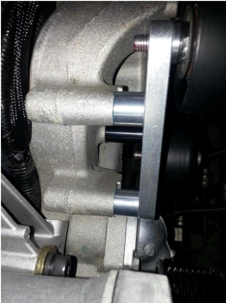
The two bolts main bolts (use RED loctite) on the top are torque to 32 ft. lbs. The 'water pump' bolt is torque to 19 ft. lbs. USE BLUE loctite on the water pump bolt.
