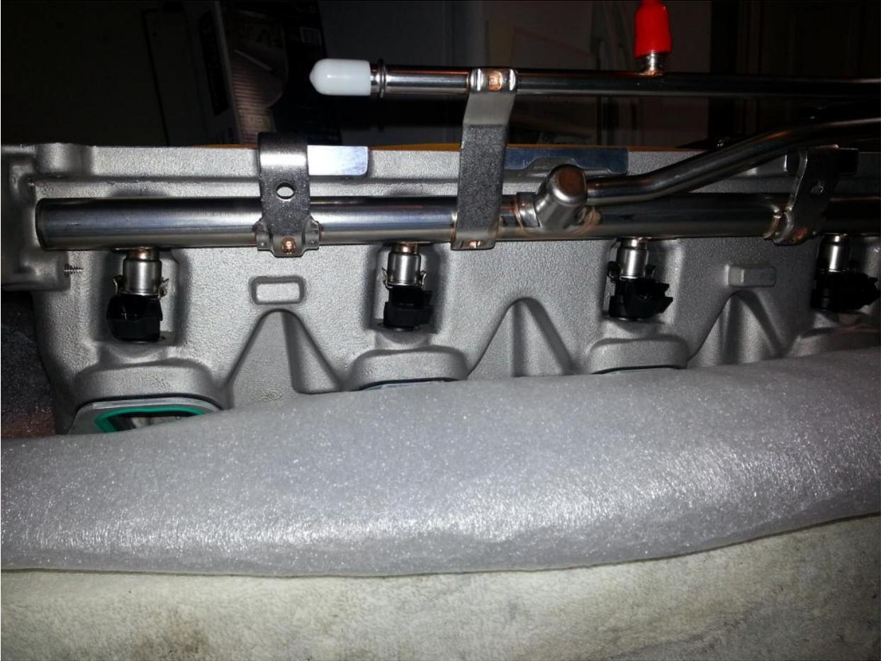
Bolted down -- NOTE leave OFF the very front bolt on the fuel rail – you will have issues with removing the fuel rail should you need to while the 'lid' is on (the picture does show it on, but it was ONLY for show):
