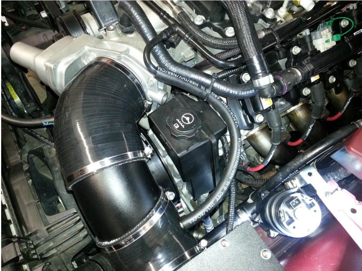
Now is the time to review and verify all vacuum lines, connectors, fuel lines, belts, spark plugs and wires, coil packs, and hoses are connected. Verify NO leaks. It is best to re-install the front wheels, place the car on the ground, and use tire blocks before starting.
