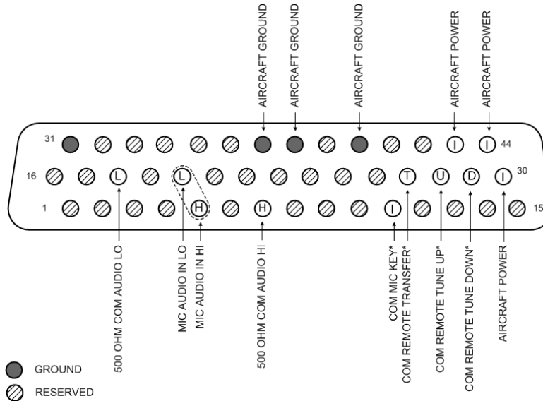
Figure A-4 J3552 Connector Layout
