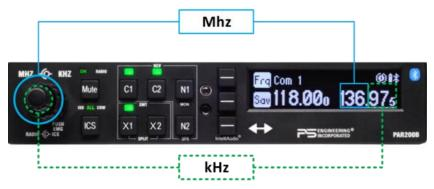
Adjust the radio and intercom volume for a comfortable listening level. Most general aviation headsets today have built-in volume controls; therefore, volume also can be further adjusted at the individual headset.
