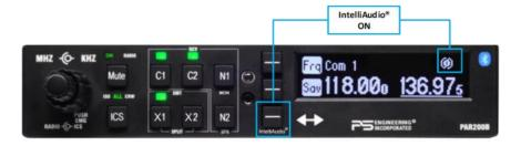
To activate the IntelliAudio HRTF mode, press and hold the bottom line-select button next to the transfer arrow for about 1 second, until the icon appears. Intercom and other audio is not spatially processed, only the pilot and copilot VHF COM audio.
