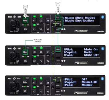
switch (J2 pin 22) to place in all heads. the passengers using the rear connector control. The streamed Bluetooth music in the PAR200B is also Music 1.
